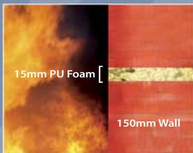
Correctly installed PU Foam
